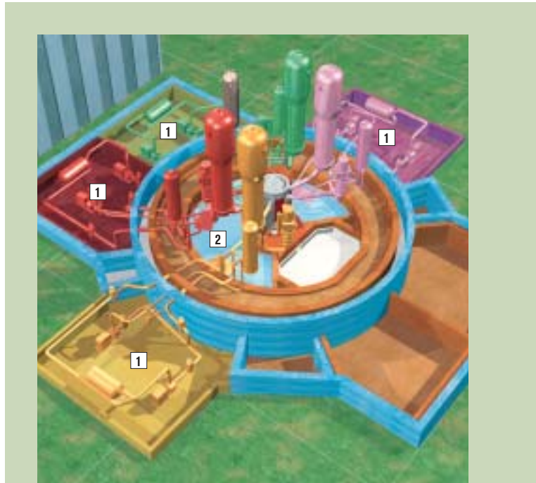
The major safety systems comprise four sub-systems or trains, each capable of performing the entire safety function on its own. There is one train in each of the four safeguard buildings (1) surrounding the reactor building (2) to prevent common-mode failure of the trains.
