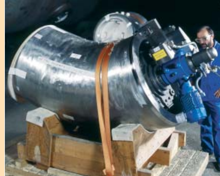
Chalon manufacturing plant (France): machining of primary piping elbow.
