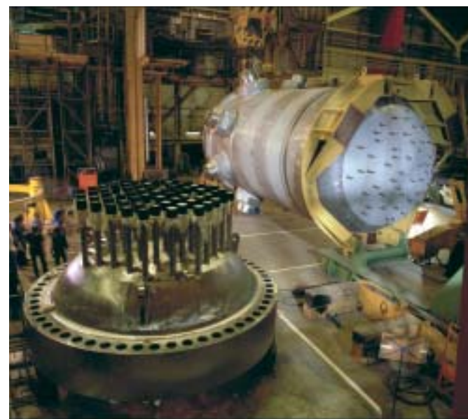
Chalon manufacturing plant (France): Civaux 1 (N4, 1,500 MWe) reactor pressure vessel and its closure head.
