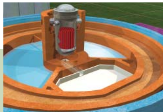
In the event of core meltdown, molten core escaping from the reactor vessel would be passively collected and retained, then cooled in a specific area inside the reactor building.
